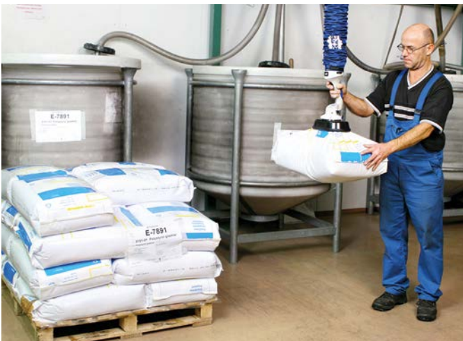
Vacuum tube lifter JumboFlex for palletizing plastic bags
