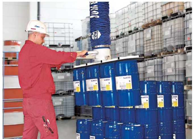
Vacuum tube lifter JumboErgo with an area gripper for handling four barrels at once
