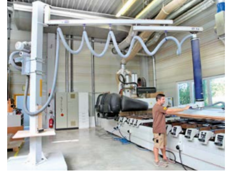
Telescopic jib for confined working areas
