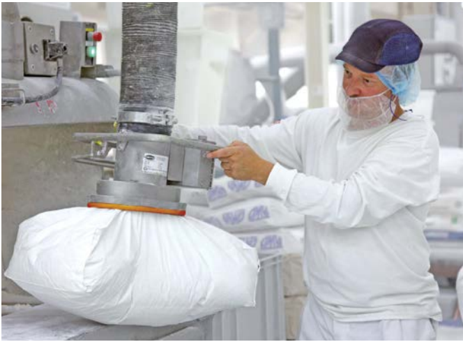
Vacuum tube lifter JumboSprint Ex for handling bags in an explosion protection zone
