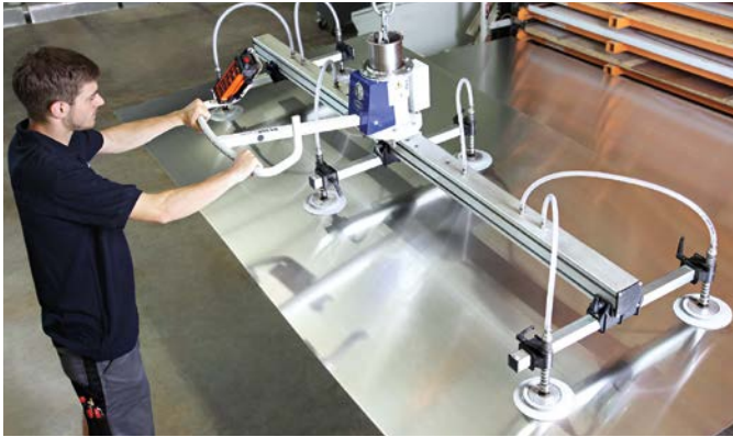
VacuMaster Eco for removing steel sheets from a drawer shelving system
