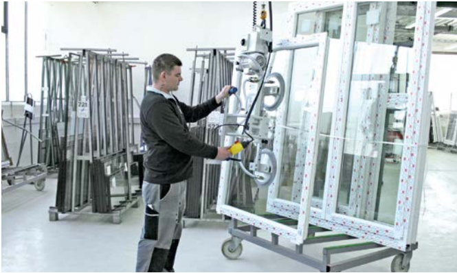
VacuMaster Window for rotating and palletizing windows
