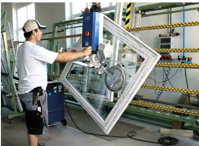
Vacuum lifting device VacuMaster Window Comfort for loading and unloading a glazing press
