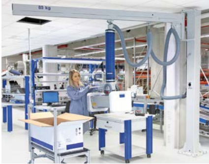
Flat jib for particularly low ceilings
