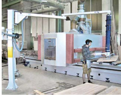
Articulated-arm jib to move around obstacles
