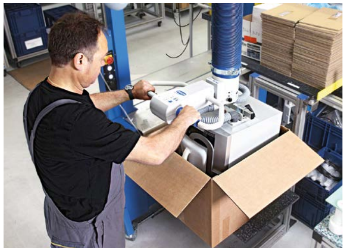
Vacuum tube lifter JumboErgo for packaging goods into boxes and handling the sealed boxes
