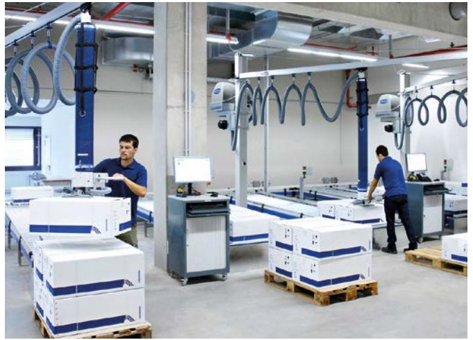
Vacuum tube lifter JumboErgo for lifting cardboard boxes
