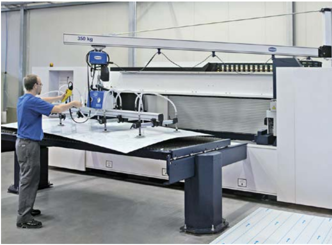
Vacuum lifting device VacuMaster Basic for loading and unloading a laser cutting machine
