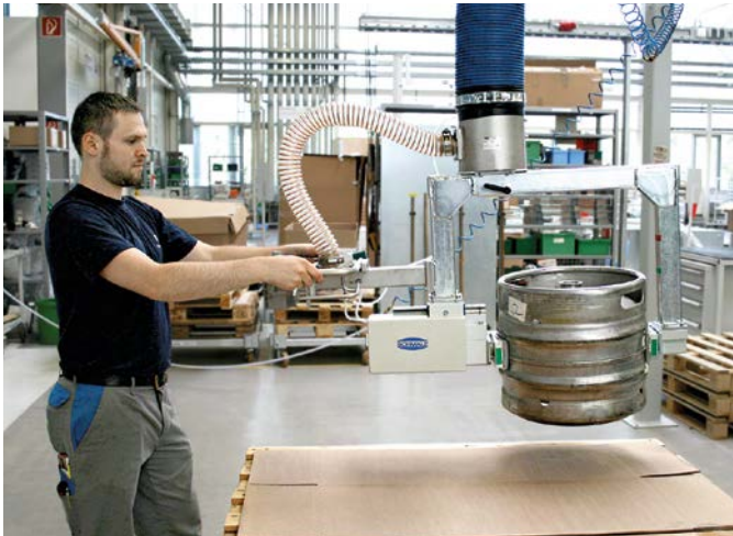
Beverage industry | Vacuum tube lifter JumboErgo with mechanical pneumatic grippers for lifting and turning kegs
