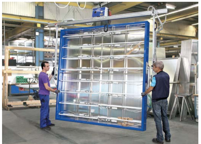
Custom solutions | Vacuum lifting device VacuMaster Box employed in the assembly of large advertising signs
