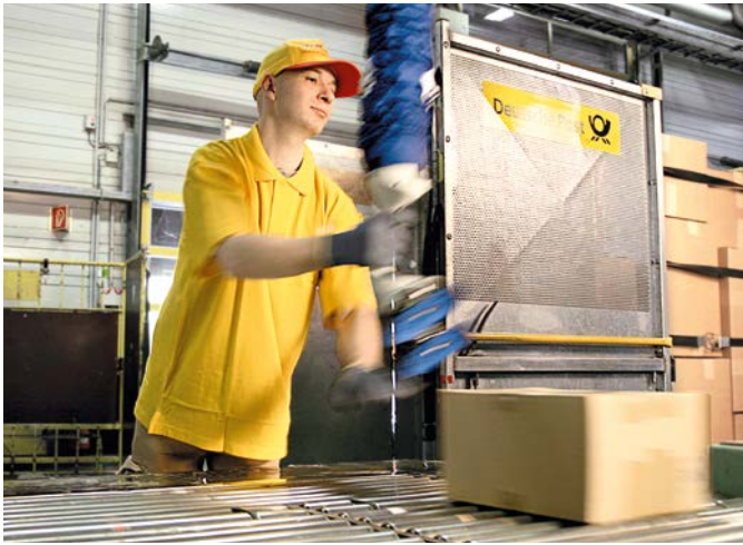
Vacuum tube lifter JumboFlex for lifting packages and for loading sorting and distribution machines
