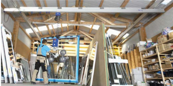
Aluminum crane system SRA with a chain hoist and vacuum lifting device VacuMaster
