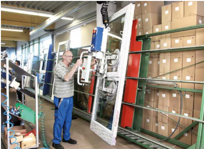
Vacuum lifting device VacuMaster Window Comfort for vertical handling of a multi-sash window
