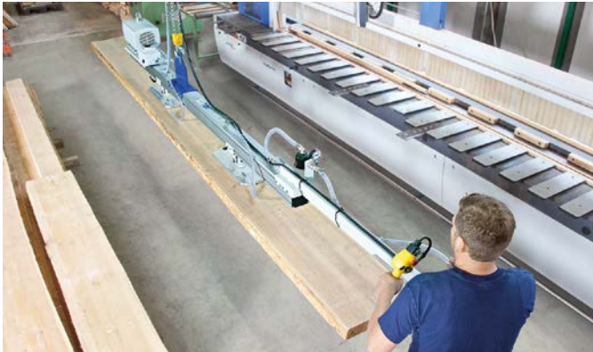
VacuMaster VHB in process of loading a rip saw with wooden boards
