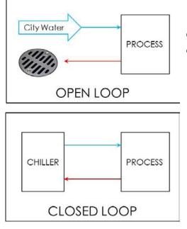
Open loop systems use cooling water to pass through a heat exchanger or directly cool and then dump the cooling water.
